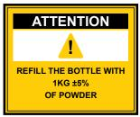
As extinguishing agent, use only the extinguishing powder mentioned in Part 4 of the label (cfr following image). Example of a fire extinguishing marking to EN3-7:2008 norm to underline the extinguishing agent reference on the label.
